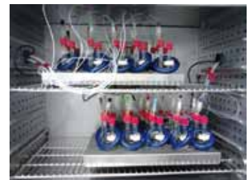
Transdermal Cells in Climate Chamber
